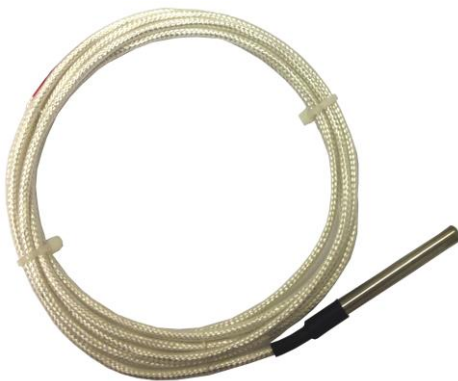
RTD: Ultra low temperature (less than -30C)
